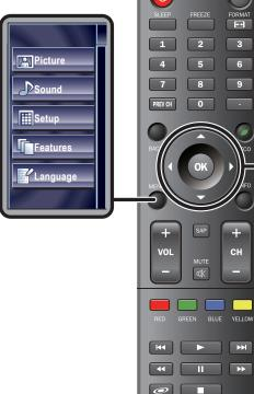
2 Use ▲/▼ to select a desired menu and an item, then press OK to determine the setting.
