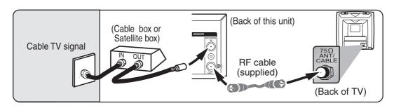
This connection allows you to view or record a scrambled channel. With this connection, channels cannot be changed on this unit. You can view or record ONLY the channels you have selected on the cable box or the satellite box.
